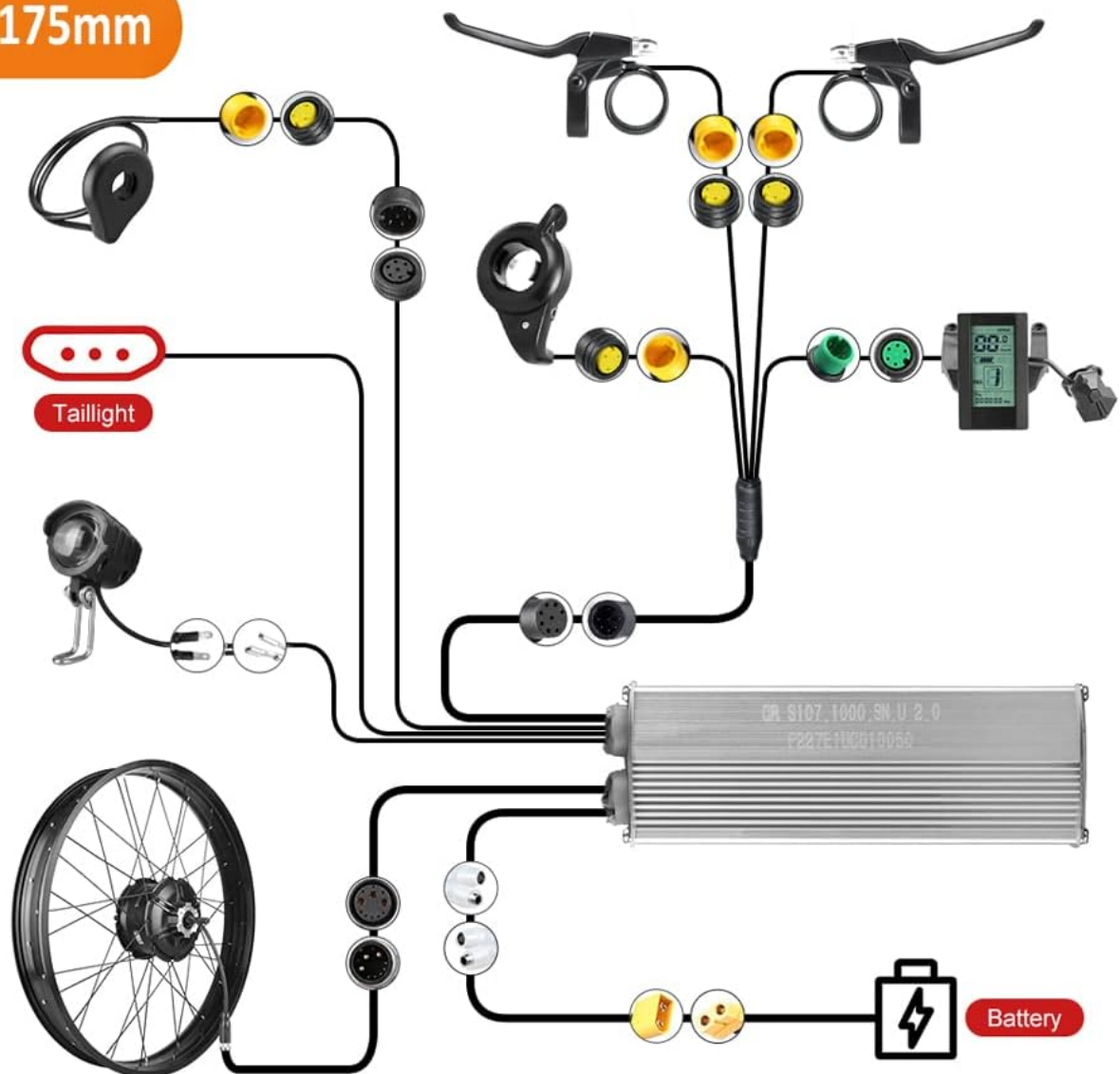
Figure 5.1: Wiring diagram for the BAFANG kit with 175mm OLD (Over-Locknut Dimension) dropout, showing connections for motor, controller, display, brake levers, throttle, PAS sensor, and battery.
