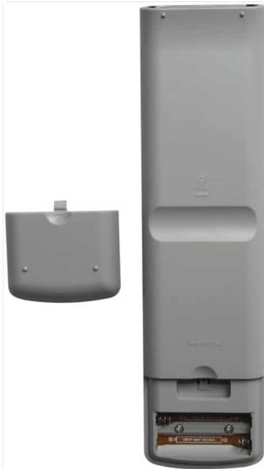
Image 2.2: The remote control with the battery cover removed, showing the correct orientation for AAA battery insertion.
