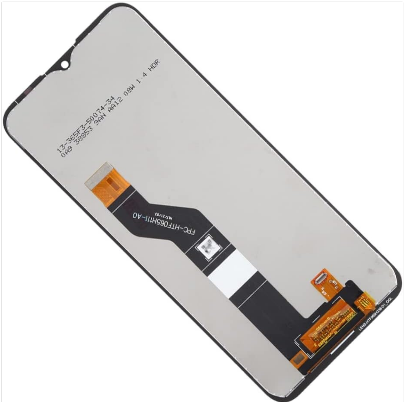
Image: Rear view of the LCD screen replacement, showing the flex cables that connect to the phone's motherboard. These cables must be handled with care during testing and installation.
