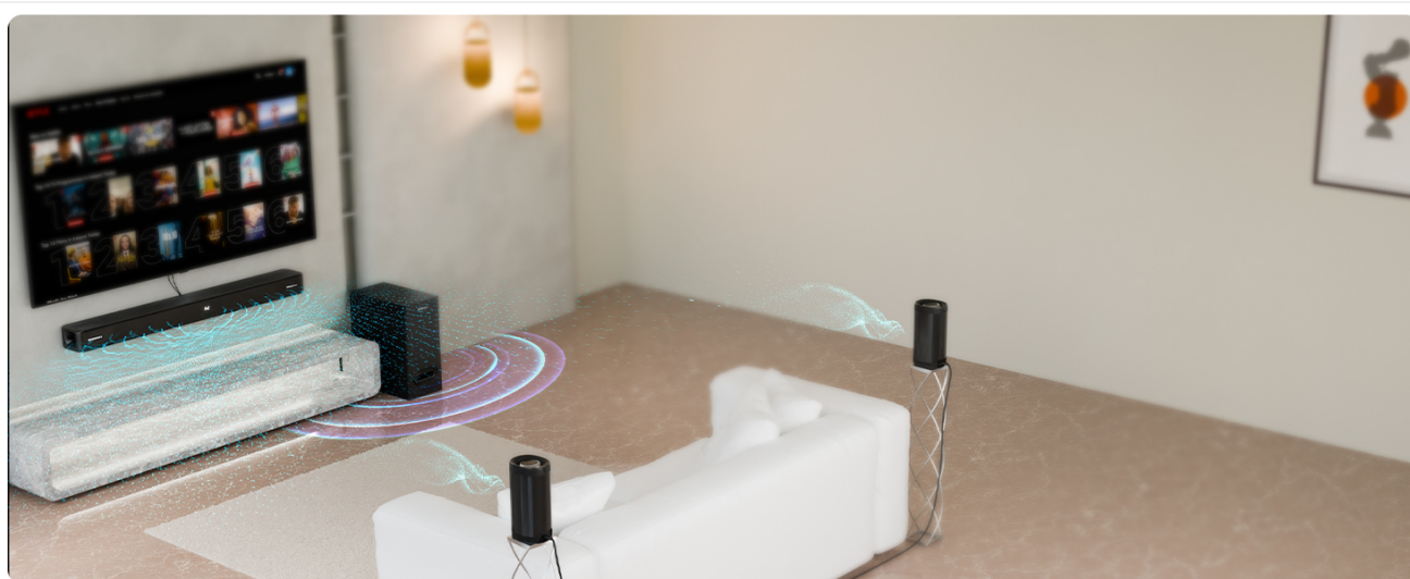
Figure 2: Visual representation of the 5.1.2 channel surround sound setup with overhead effects from Dolby Atmos.
