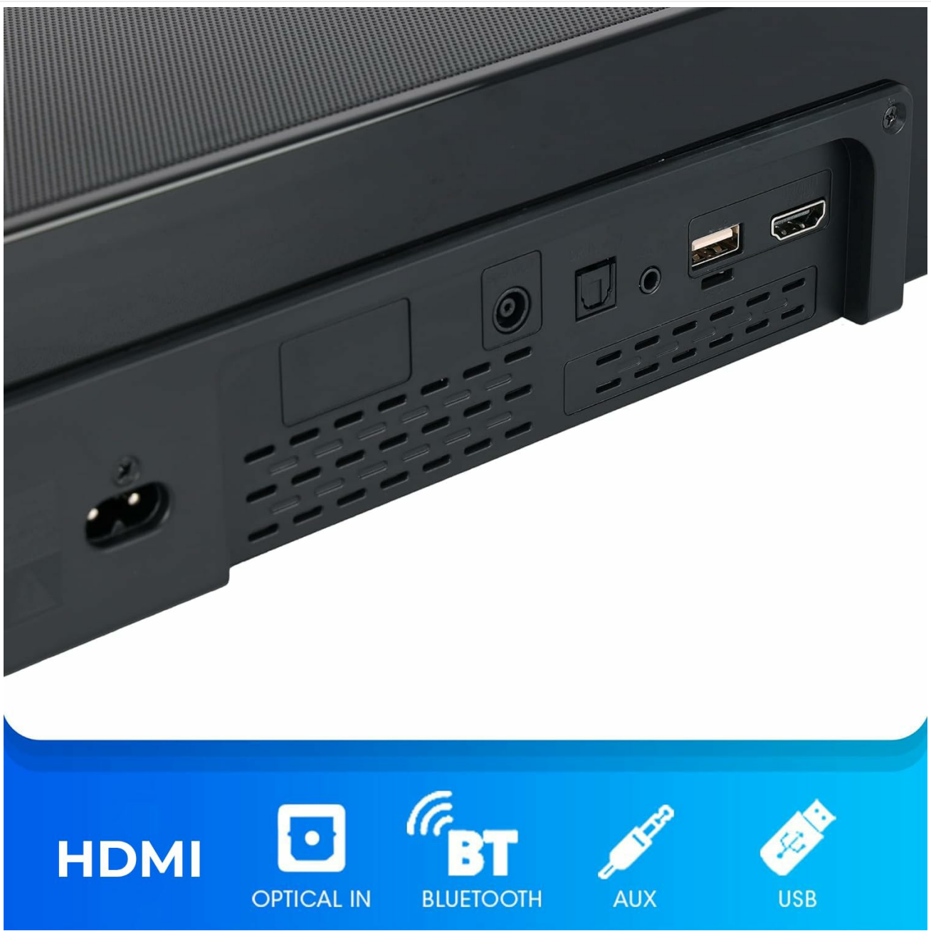
Figure 4: Close-up view of the soundbar's rear panel with HDMI eARC, Optical, AUX, and USB input ports.
