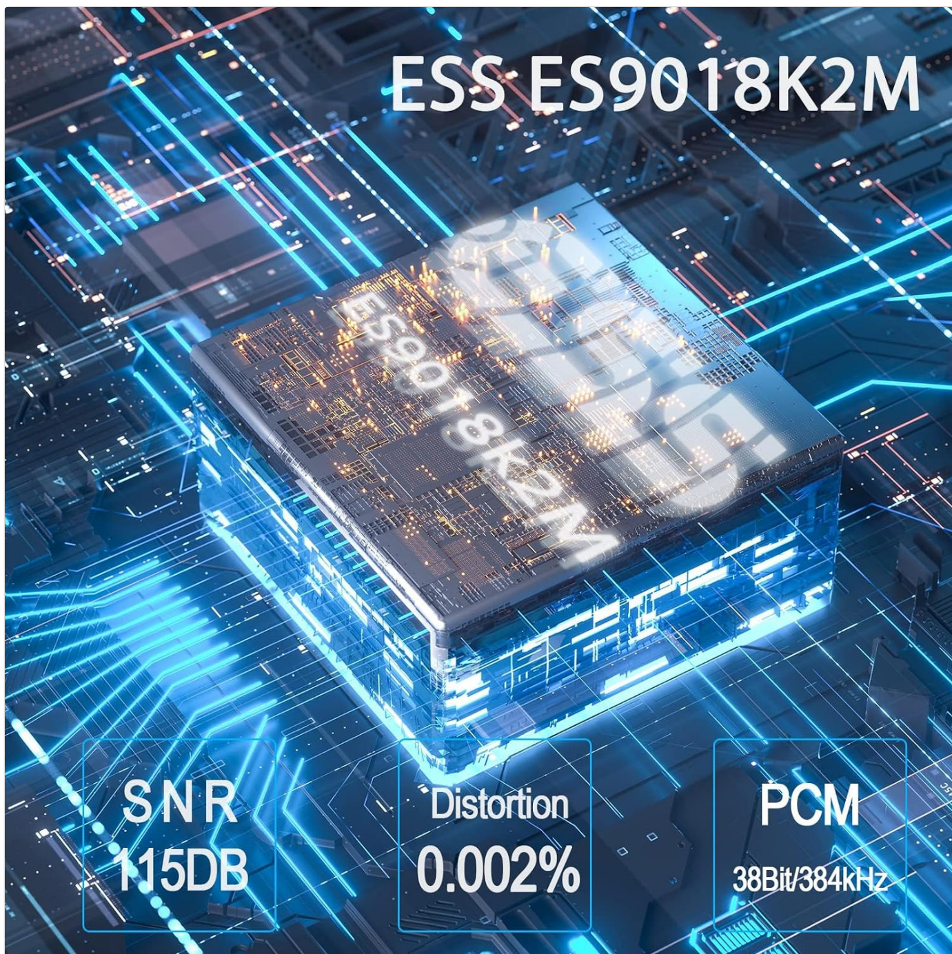
Image: A detailed view of the ESS ES9018K2M audiophile-grade DAC chip, highlighting its role in providing high-quality audio with specifications like 115dB SNR, 0.002% distortion, and 38Bit/384kHz PCM support.
