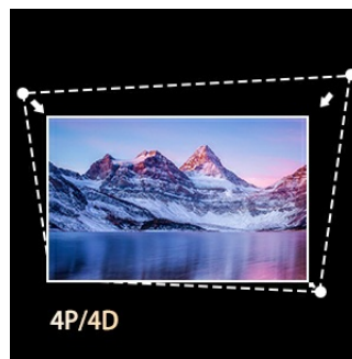
Image: Diagram showing how 4P/4D keystone correction can be used to adjust the corners of a projected image to achieve a rectangular shape.
