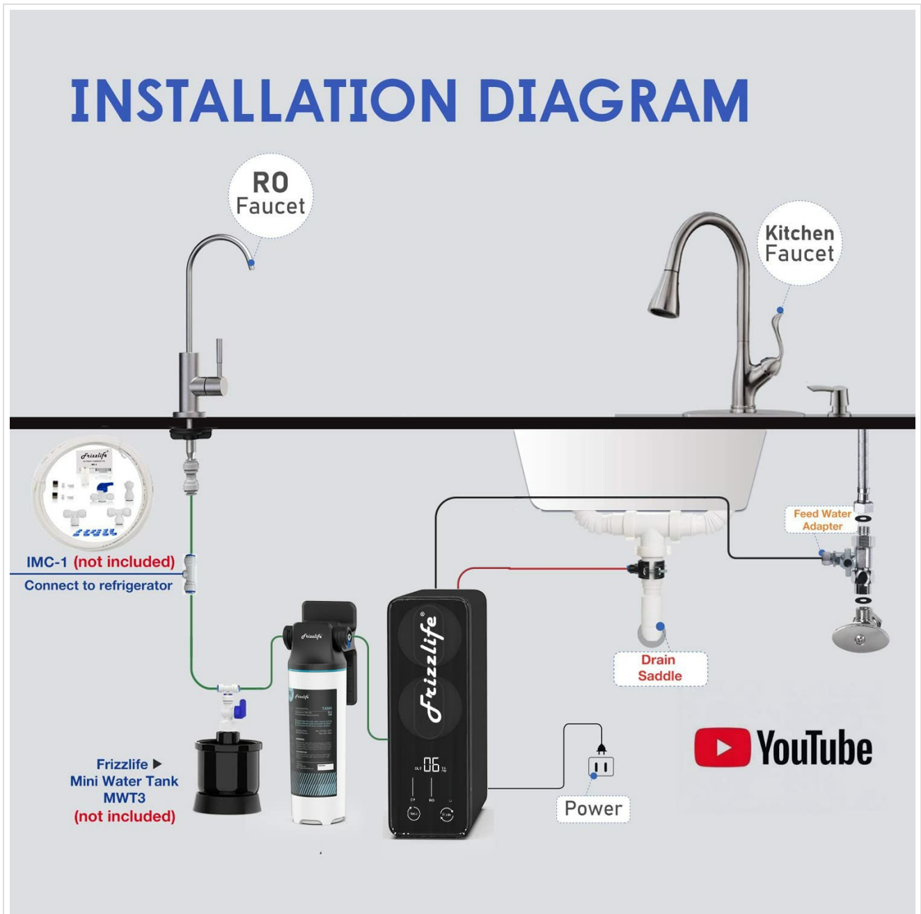
Figure 3.1: An overview of the Frizzlife PD1000-TAM4 system installation, showing connections to the RO faucet, kitchen faucet, feed water adapter, drain saddle, and optional ice maker kit.
