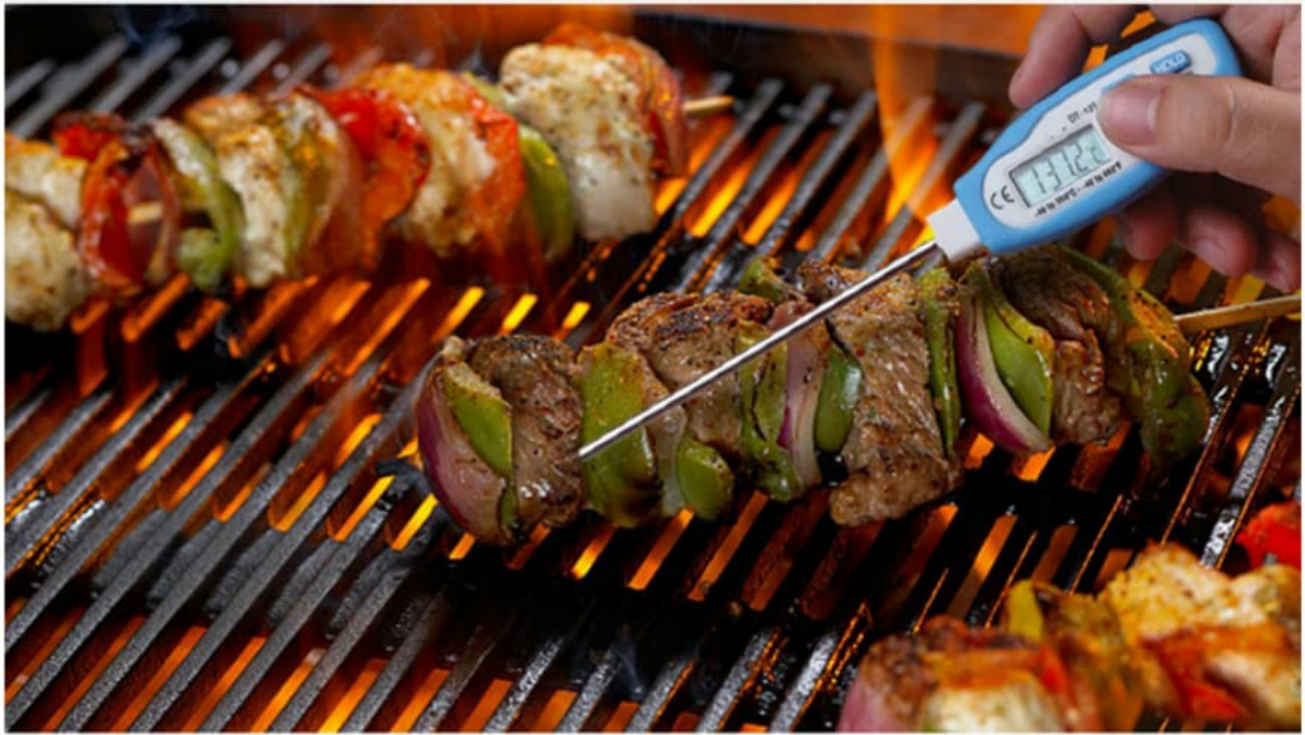
Image: The DT-131 thermometer being used to measure the internal temperature of food on a grill.
