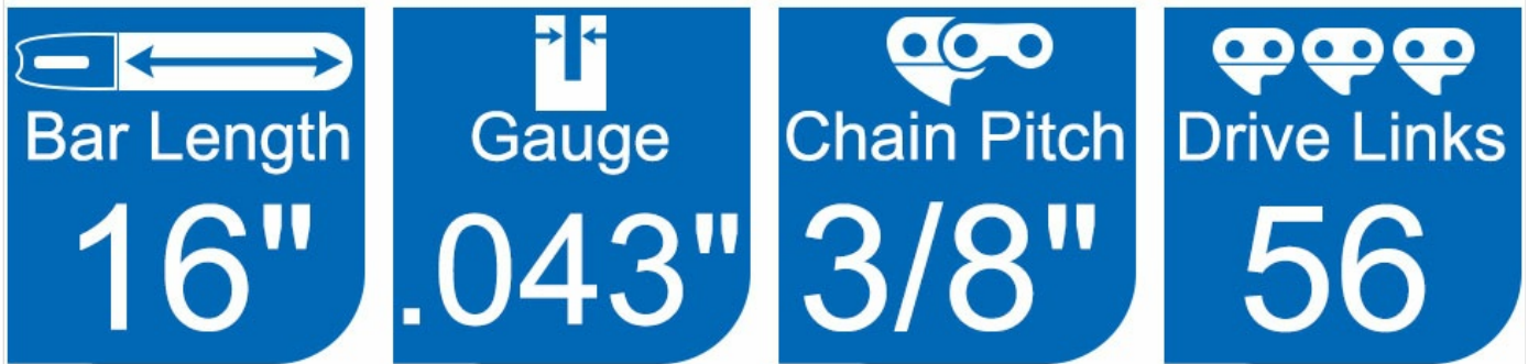
Image 3.2: Key parameters for chainsaw chain compatibility. Ensure your chainsaw matches these specifications.
