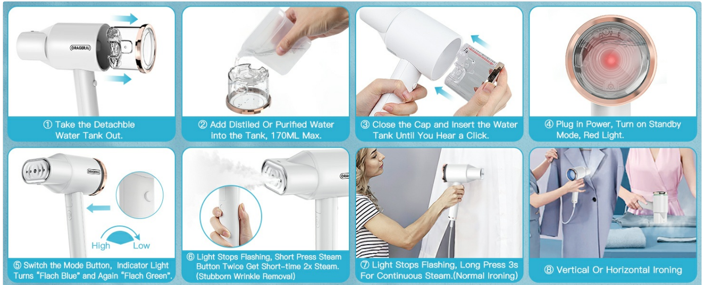
Figure 2: Visual guide for preparing and using the steamer.
