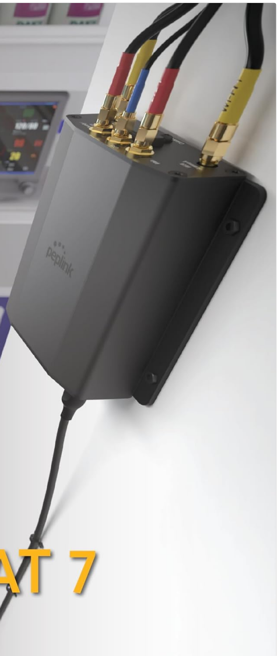
Figure 3.1: Front view of the Peplink MAX BR1 Mini CAT-7 router with four LTE antennas connected.
