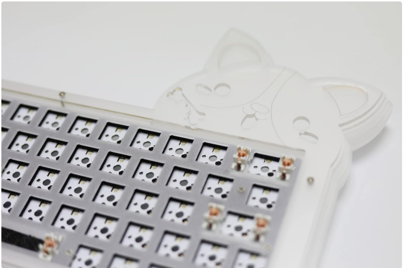
Image: The keyboard kit's PCB and plate, showing the hot-swappable sockets where mechanical switches are to be inserted. The puppy head design is visible on the right.
