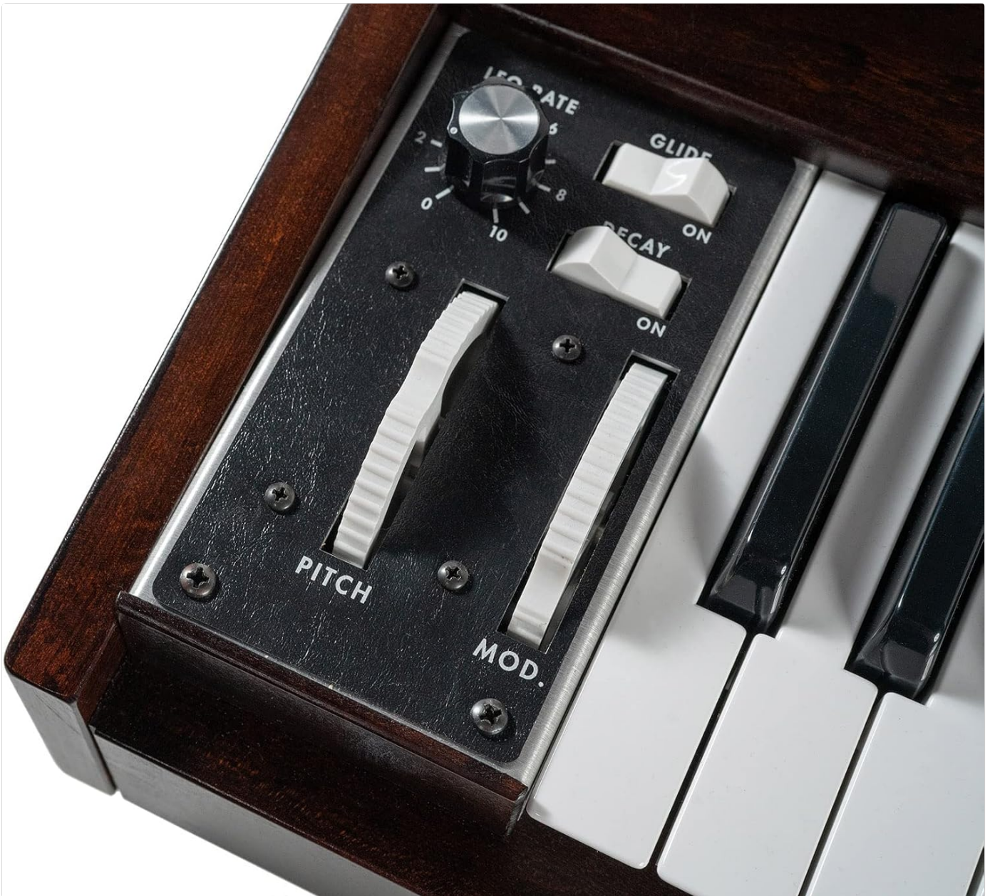
Close-up view of the Minimoog Model D's iconic pitch bend and modulation wheels, along with the LFO rate, glide, and decay controls.
