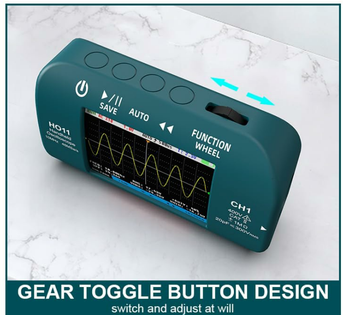
Figure 3.3: Close-up views highlighting the save button for capturing images, the integrated foldable stand for hands-free operation, the convenient Type-C charging port, and the gear toggle button for easy adjustments.
