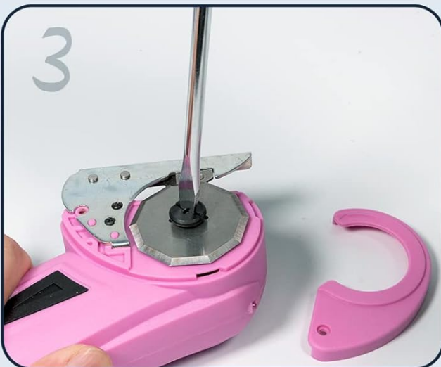
3. Unscrew the screw holding the blade in place
