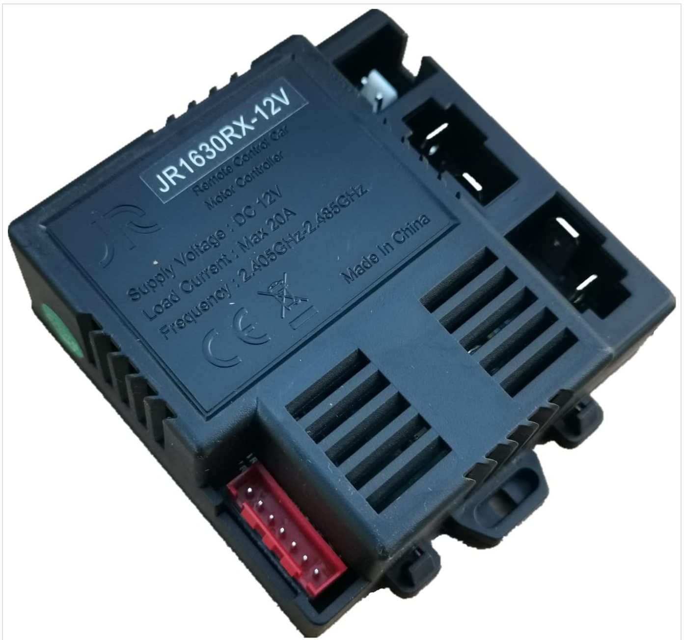
Image 2: Angled view of the FULIHUAPOW JR1630RX-12V Control Box Receiver, highlighting its compact design and connectors.
