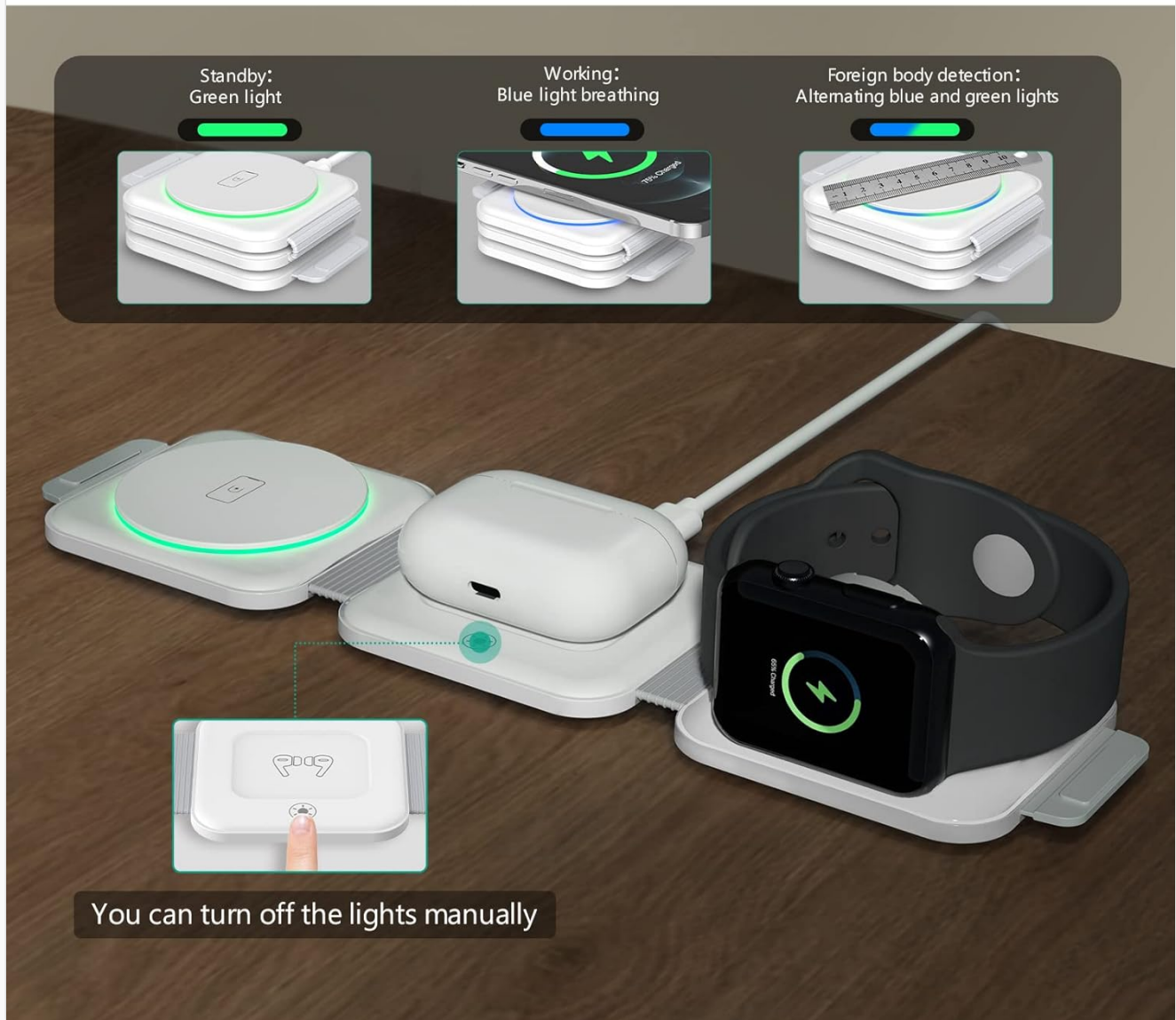
Image 6.1: Visual representation of the charging indicator light's different states and their meanings.
