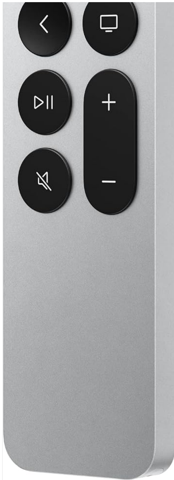
Image 1: Front view of the Apple TV Siri Remote (3rd Generation), showing the clickpad, menu, TV, play/pause, volume, and mute buttons, along with the power button at the top.
