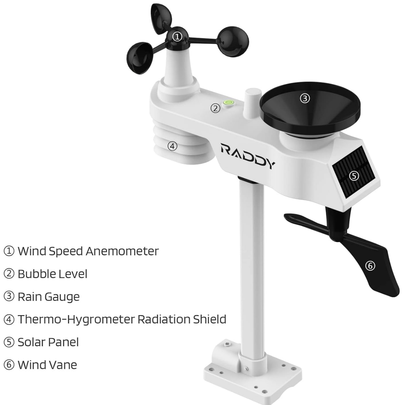
Image: Components of the Raddy WF-100C Lite outdoor sensor with labels.
