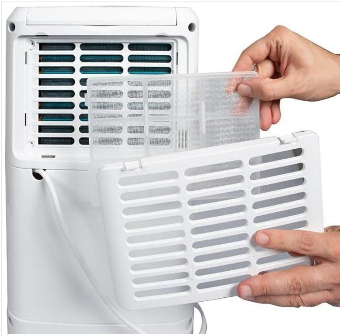
Figure 5.2: Hands removing the air filter from the Habitex H1000 Dehumidifier. This image shows how to access and detach the washable air filter from the back of the unit.
