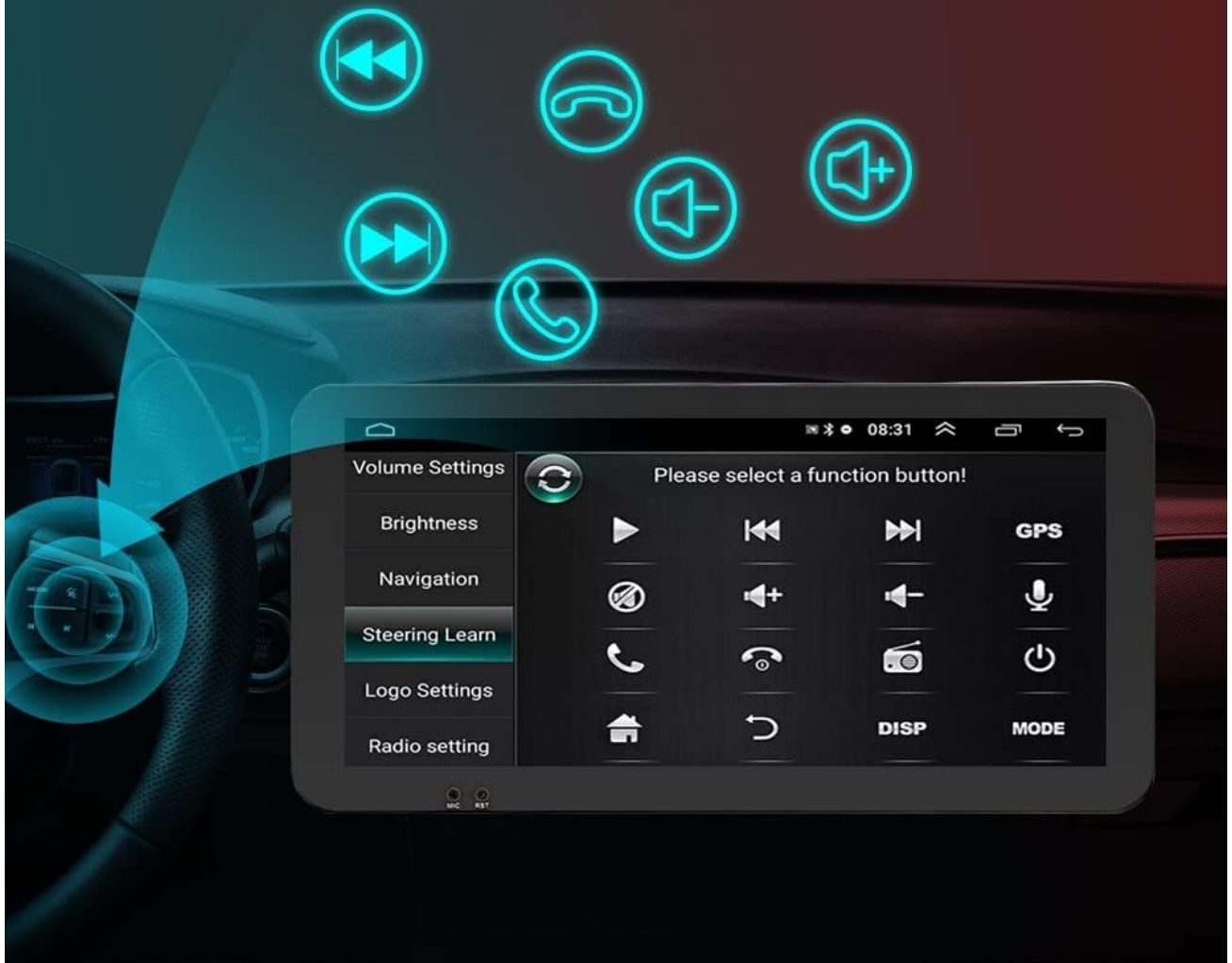
Image 3.5: Interface for configuring steering wheel controls, showing various assignable functions.
