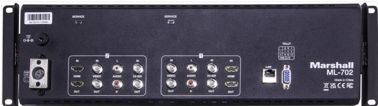
Figure 2.1: Rear panel of the ML-702 monitor, illustrating the various input and output connections for video, audio, and power, including HDMI, 3G-SDI, CVBS, and LAN ports.
