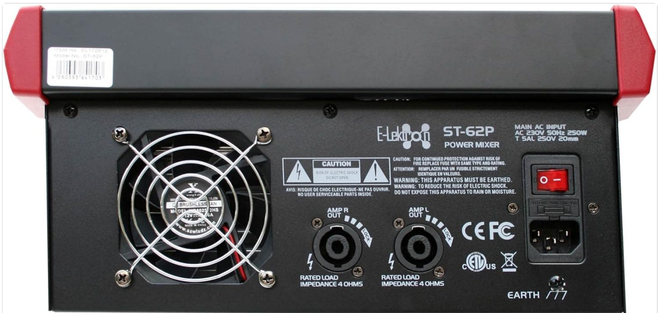
Figure 2: Rear view of the E-Lektron ST-62P, illustrating the power input, speaker outputs (AMP R OUT, AMP L OUT), and cooling fan.
