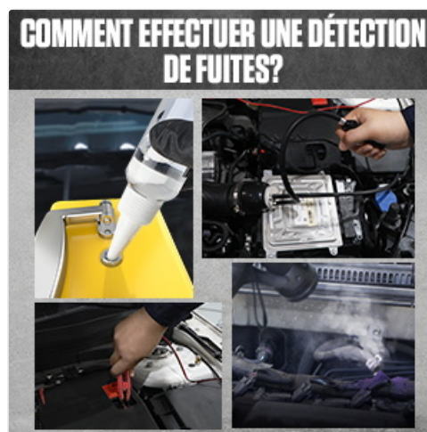
Figure 6: Visual guide on how to perform a leak detection, including adding oil, connecting power, and observing smoke.
