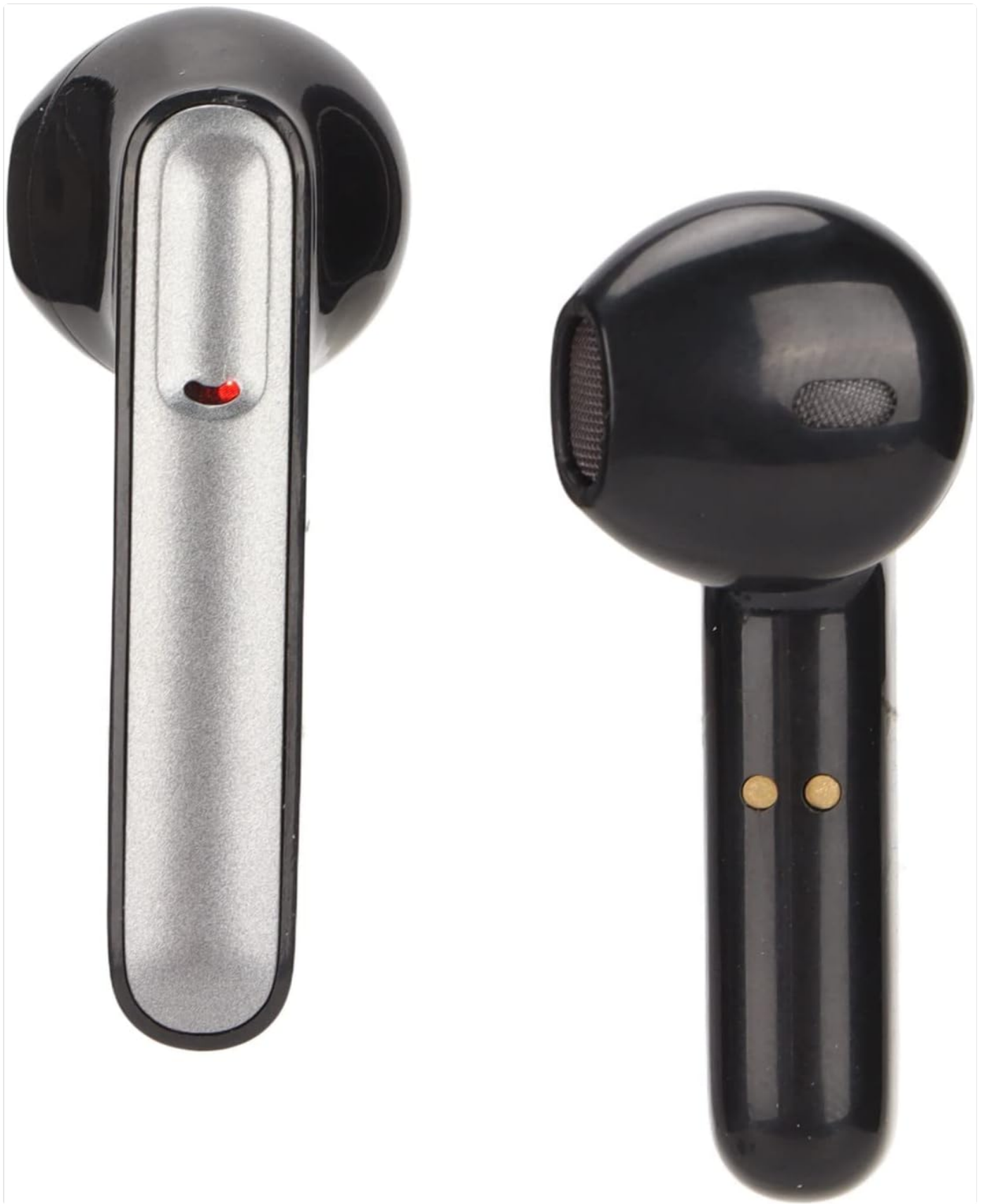
Image: Front and back views of the Septenta P40 earbuds, showing the speaker grille and charging contacts.
