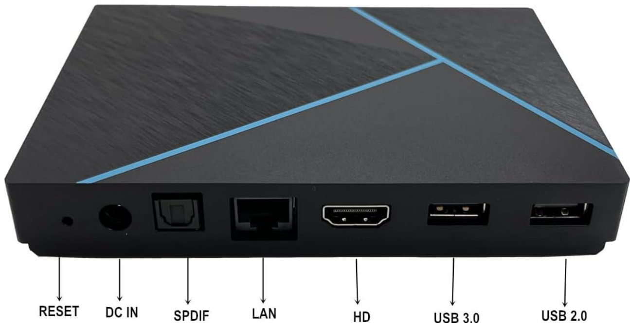
Image: Rear panel of the H96 MAX V56 TV Box showing various connection ports.
