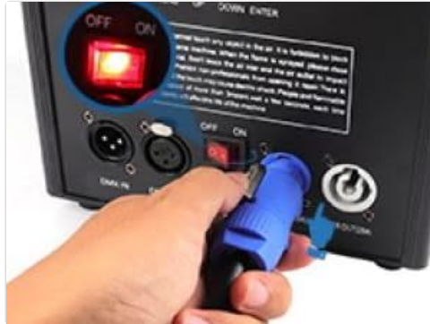
Figure 5.1: Powering On - Activating the main power switch.
