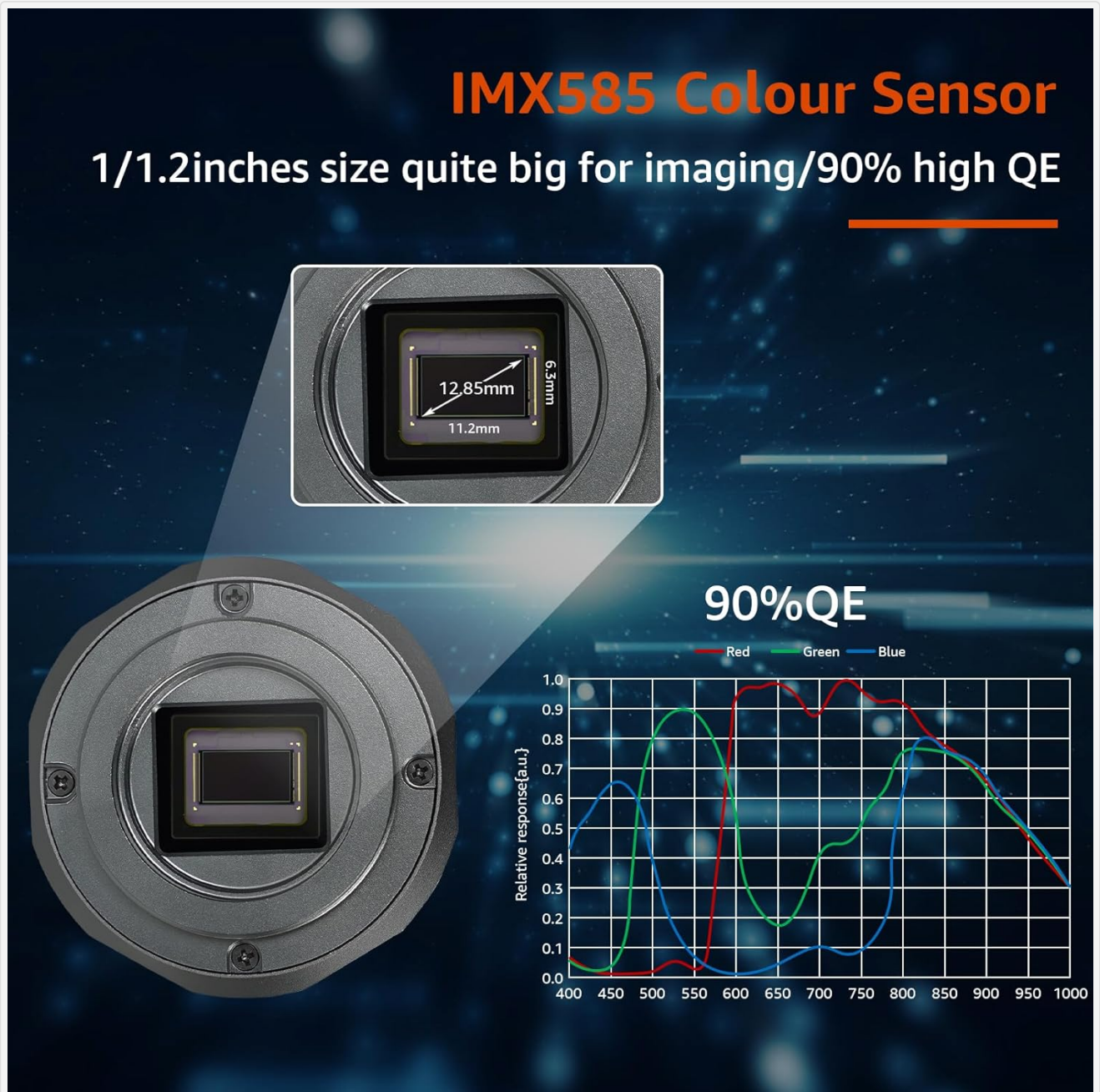
Image 3.1: Diagram illustrating the IMX585 color sensor with its dimensions and quantum efficiency (QE) curve, showing high sensitivity across visible and near-infrared spectrums.
