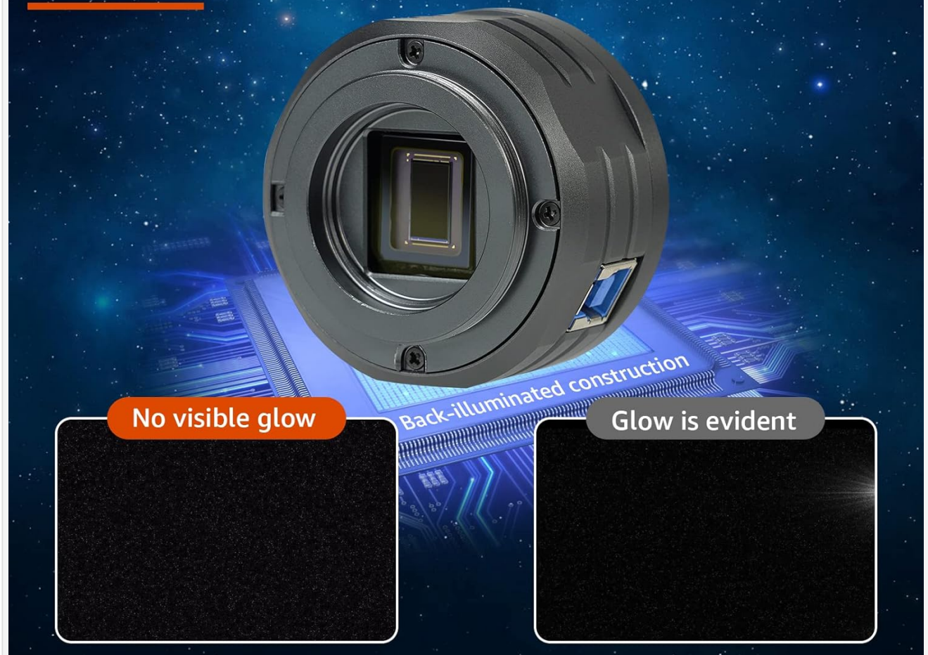
Image 3.2: Comparison demonstrating the absence of amplifier glow in images captured with the SV705C camera, resulting in a clean background.
