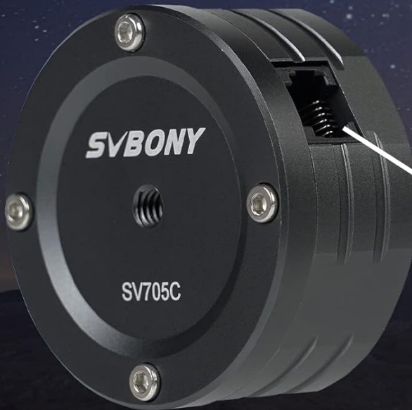
Image 4.1: Close-up view of the SV705C camera showing the USB3.0 data interface and the ST4 guided star interface for connectivity.
