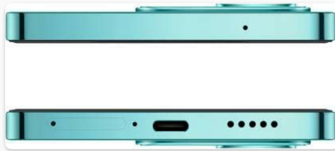
Figure 2.1: Top and bottom view of the Vivo V25 5G, highlighting the SIM tray and USB-C port.
