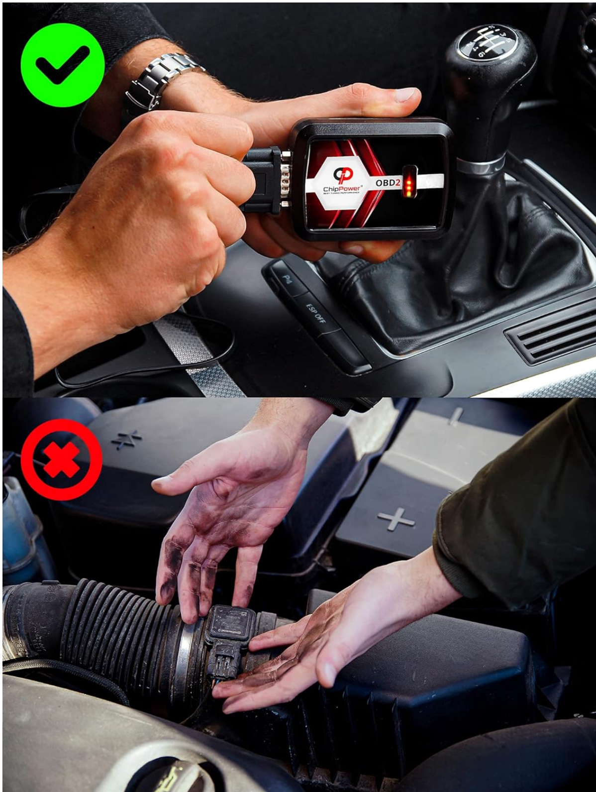
Image 5.1: Proper installation involves connecting the module directly to the vehicle's OBD port inside the cabin (top image). Avoid connecting it directly to engine components (bottom image).
