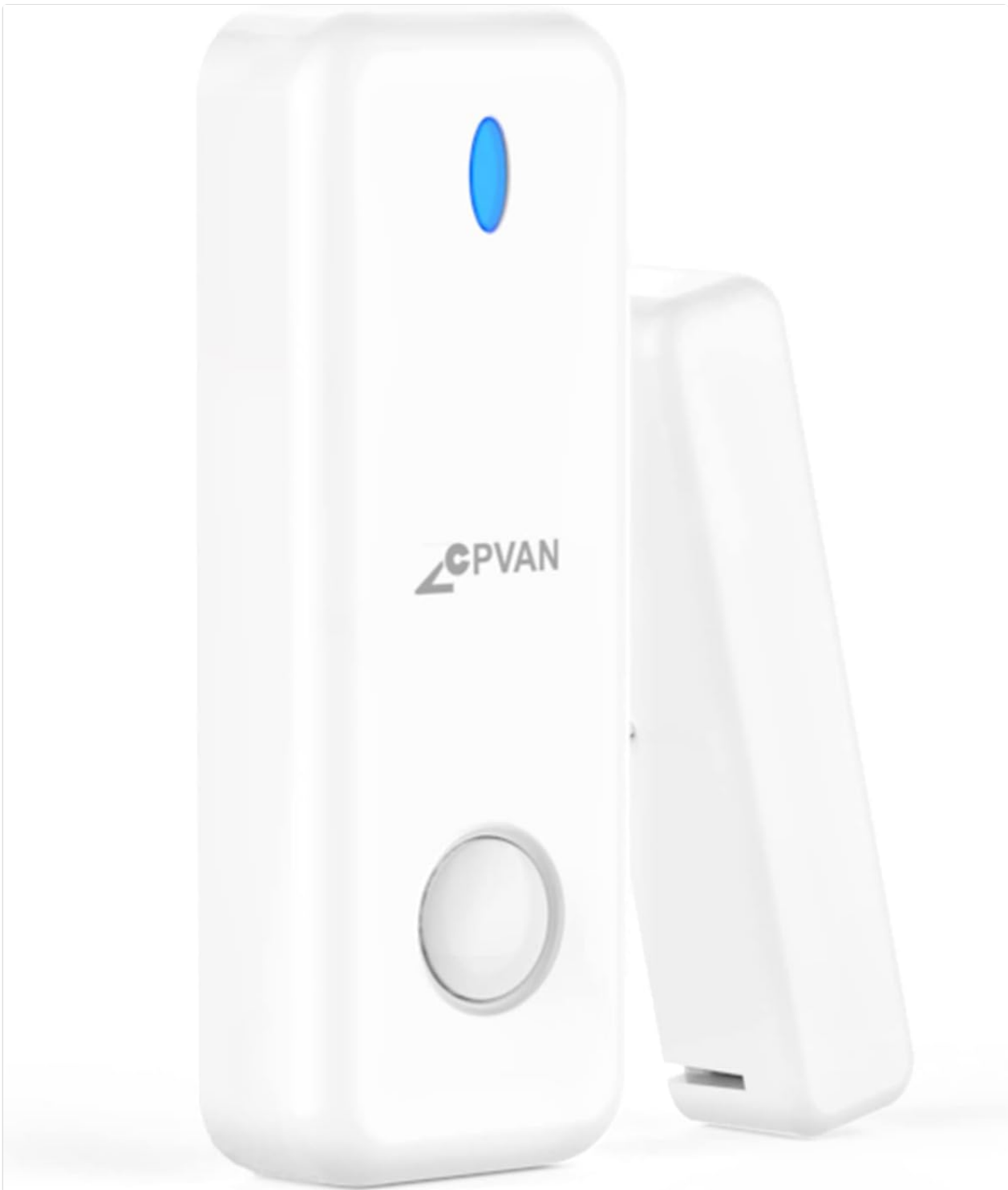
Image 1: The CPVAN CP8 Door and Window Sensor, showing the main unit and the magnetic component.
