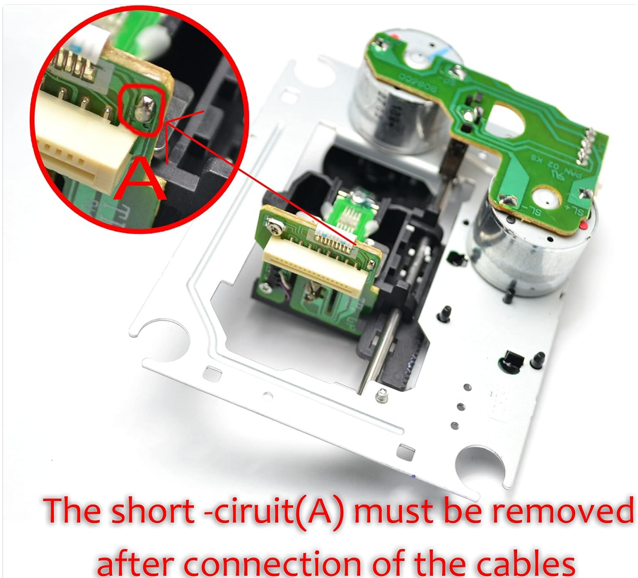
Figure 4.1: Critical step: The anti-static short circuit (A) must be removed after connecting all cables and before powering on the device.
