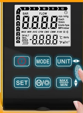
Figure 5: Close-up of the INFURIDER YF-6000GH's clear LCD backlight display and sensitive smart multi-touch screen, highlighting the 8-vane sensor. The device features a clear LCD backlight display and a sensitive smart multi-touch screen with several buttons:
