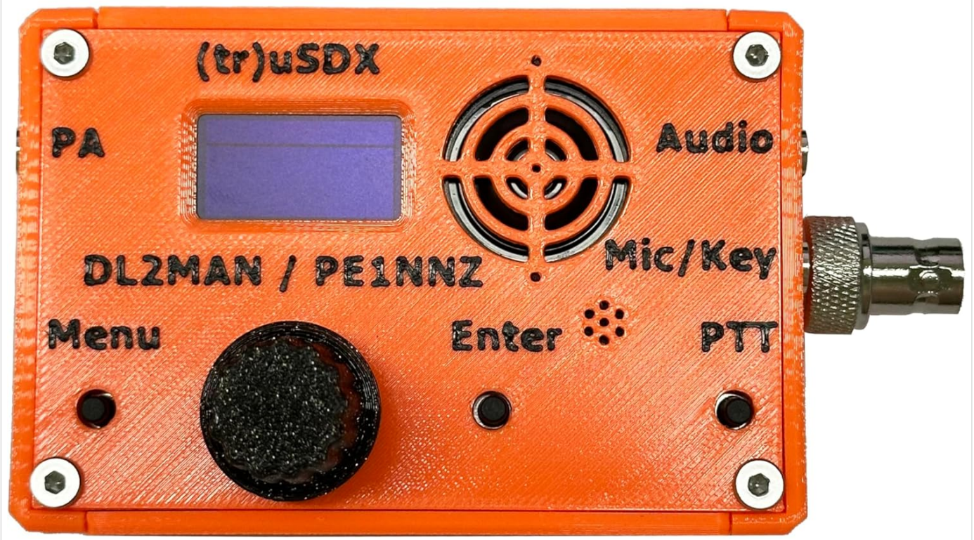
Figure 2: Front view of the Malahit tr usdx Transceiver, showing the OLED display, speaker, and control buttons.
