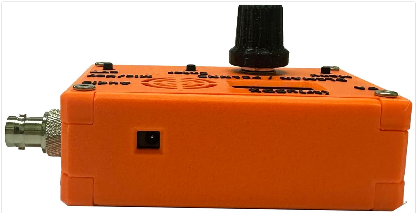
Figure 4: Side view of the Malahit tr usdx Transceiver, showing the power input port.
