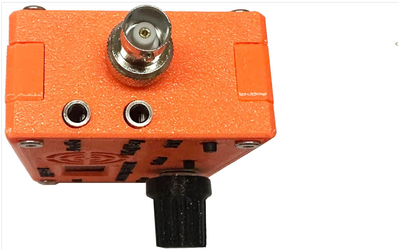
Figure 5: Top view of the Malahit tr usdx Transceiver, showing the antenna connector and other ports.
