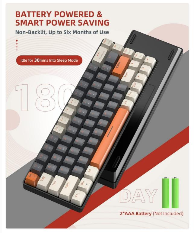
Visual representation of the keyboard's battery power and smart power-saving capabilities, including its automatic sleep mode.
