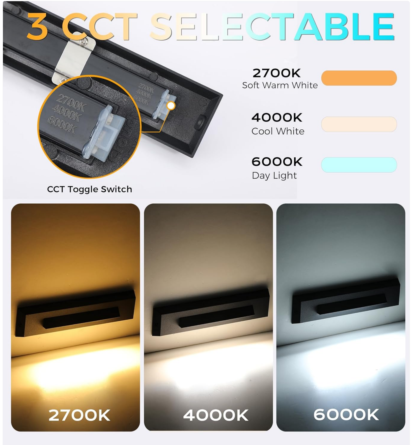
Figure 3: 3 CCT Selectable Feature. The toggle switch allows selection between 2700K, 4000K, and 6000K.
