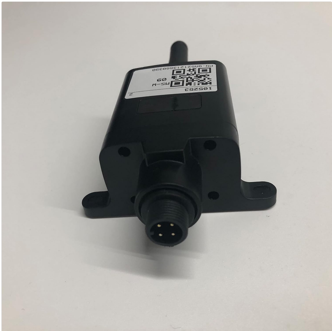
Figure 2: Bottom view of the WiFi adapter. This image shows the RS232 connector port on the adapter, which connects to the inverter.
