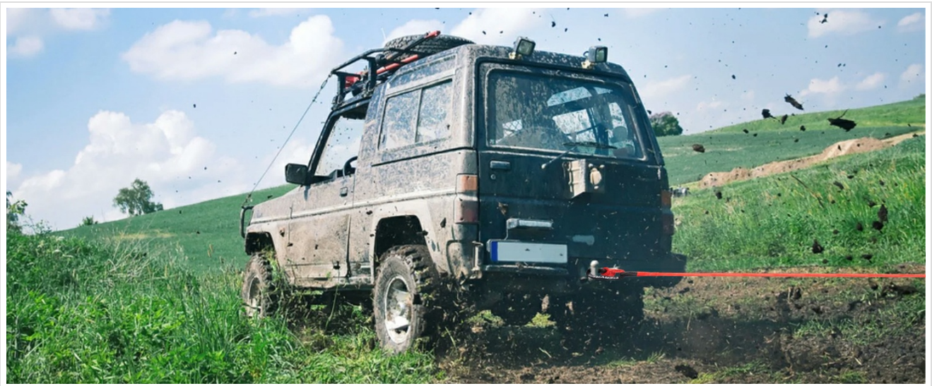
Image: A red kinetic recovery rope connecting a recovery vehicle to a stuck vehicle, demonstrating the rope's stretch during a pull.
