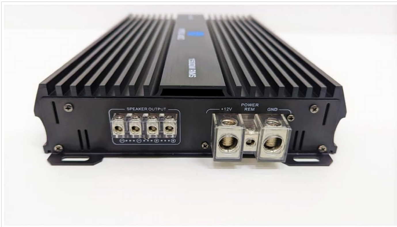
Image 2: Rear view of the amplifier, detailing the power input terminals (+12V, REM, GND) and speaker output terminals.
