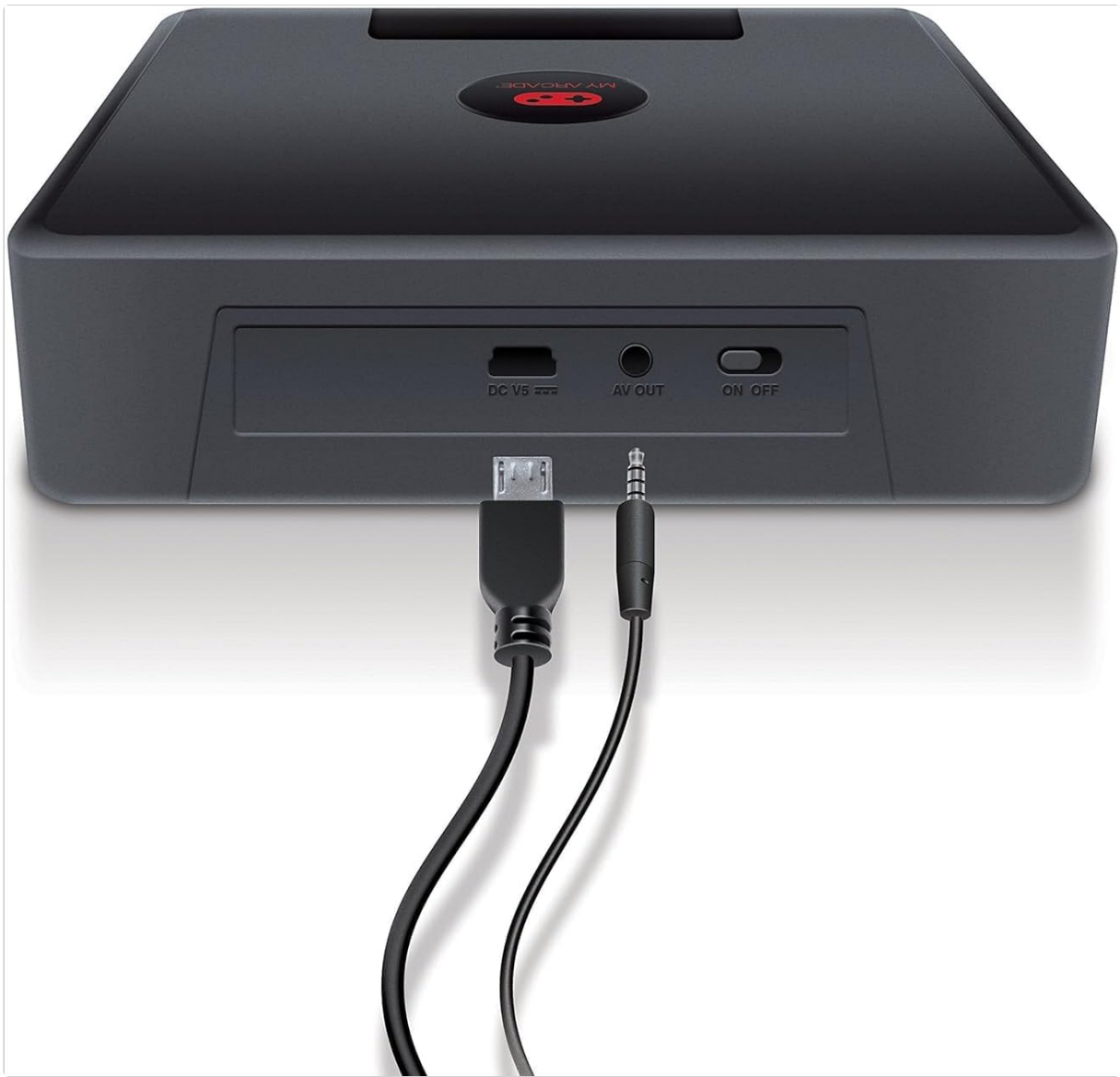
Image: Rear view of the GameStation console, highlighting the DC 5V (USB power) and AV OUT ports, and the ON/OFF switch.
