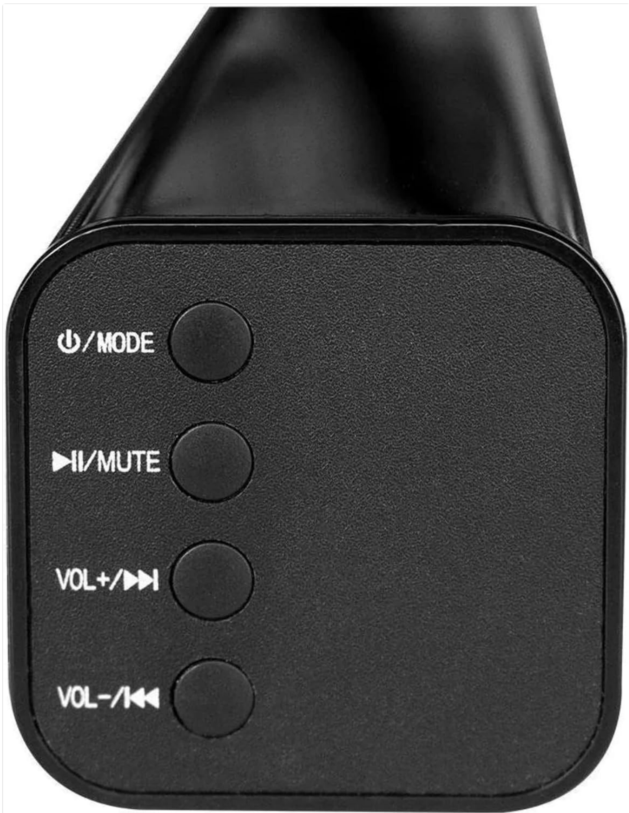
Figure 4.5: Side panel controls on the soundbar, including Power/Mode, Play/Mute, Volume Up/Next, and Volume Down/Previous buttons.
