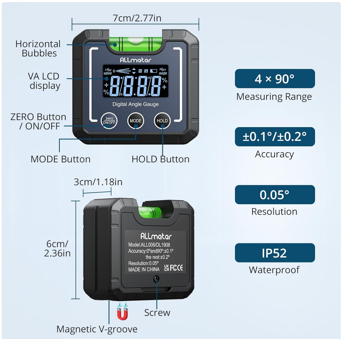
Image: A detailed diagram highlighting the Horizontal Bubbles, VA LCD display, ZERO Button / ON/OFF, MODE Button, HOLD Button, Magnetic V-groove, and screw. Key specifications like 4x90° Measuring Range, ±0.1°/±0.2° Accuracy, 0.05° Resolution, and IP52 Waterproof rating are also shown.
