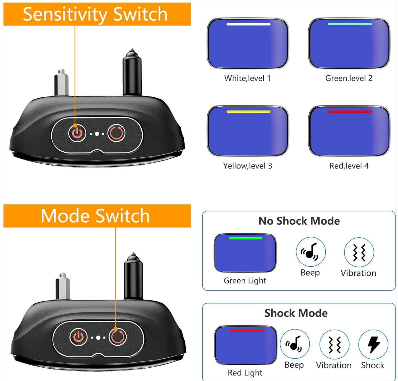
Figure 2: Illustration of the sensitivity and mode switches, detailing the indicator light colors for each setting.
