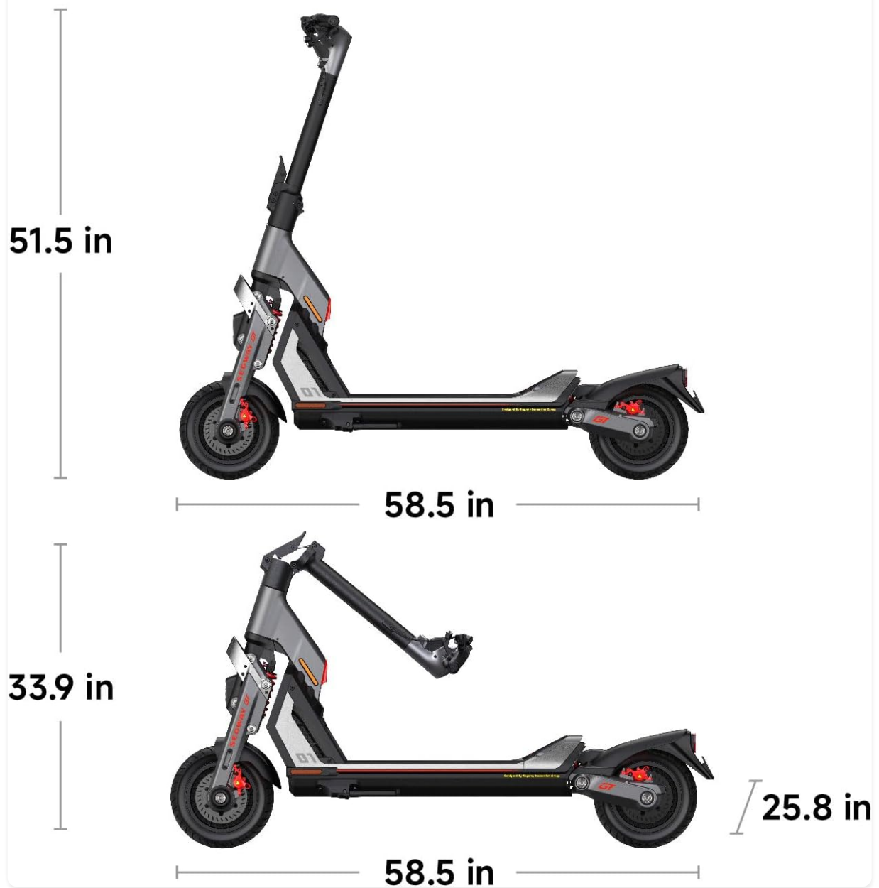
Figure 6: Dimensions of the Segway SuperScooter GT1P in both unfolded and folded states.
