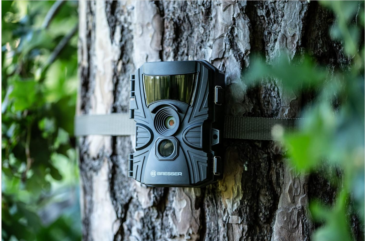
Figure 3.2: The camera securely mounted to a tree using the provided strap.
