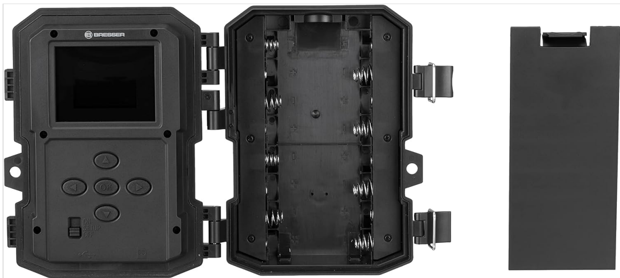
Figure 3.1: Interior view showing the control panel, screen, and battery compartment.
