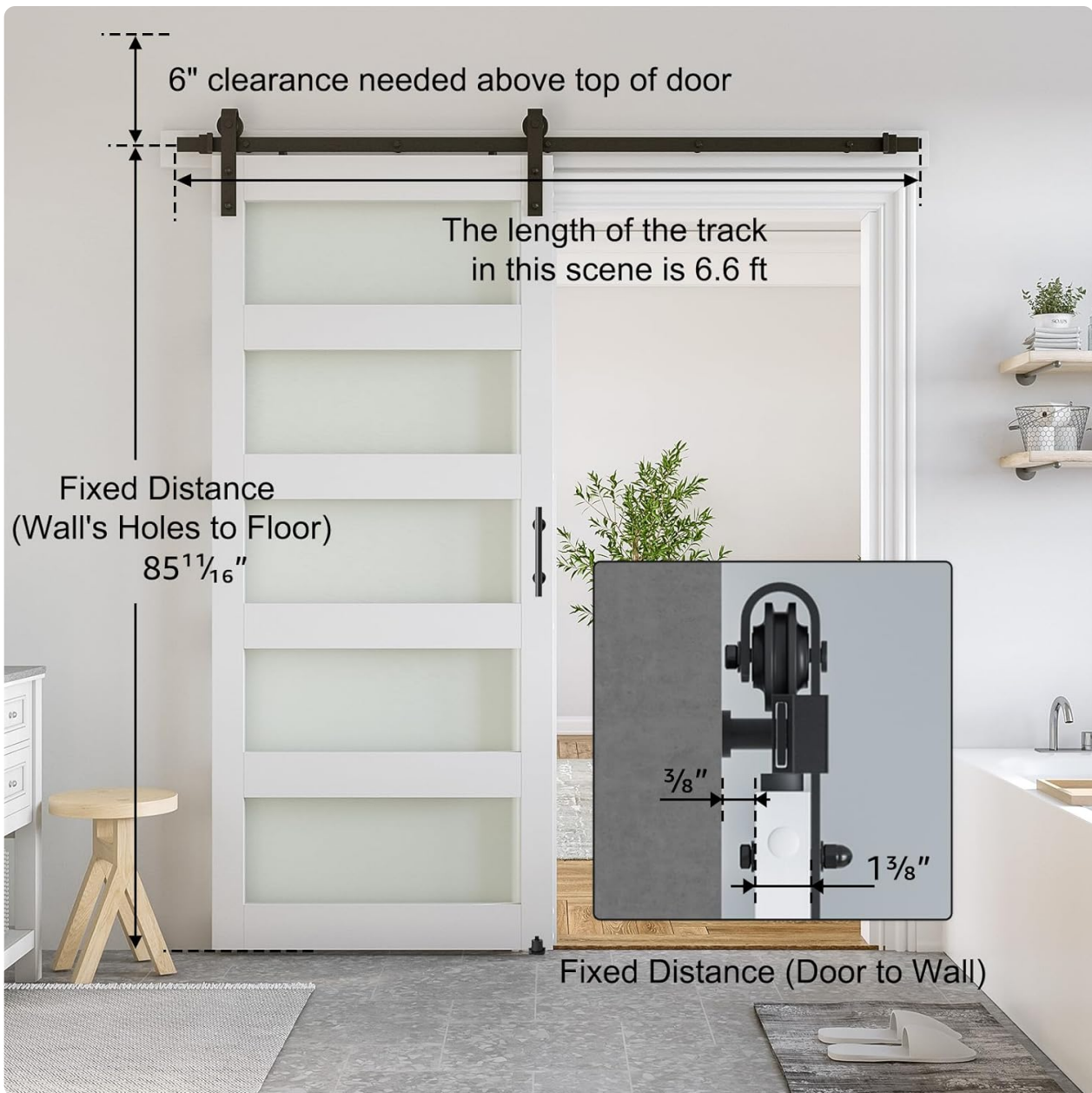
Image: Visual guide for barn door installation clearances, showing the 6-inch clearance needed above the door and the fixed distance from wall holes to the floor.
