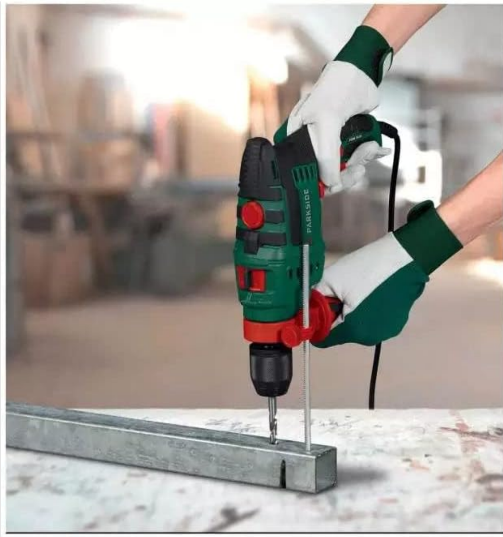
Figure 2: Drilling into a metal workpiece. This image shows a person wearing protective gloves operating the Parkside drill to create a hole in a metal beam. The depth stop is visible, indicating precise drilling.
