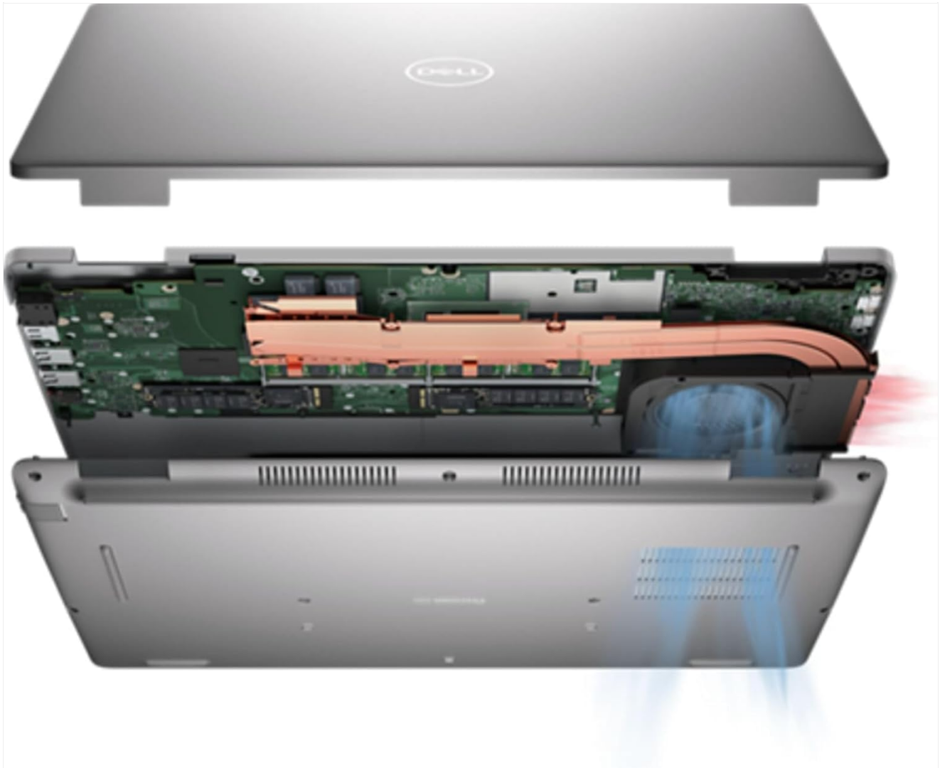
Internal view highlighting the cooling system and ventilation.
