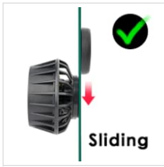
Image 5.1: Correct installation method (sliding the external magnet).
