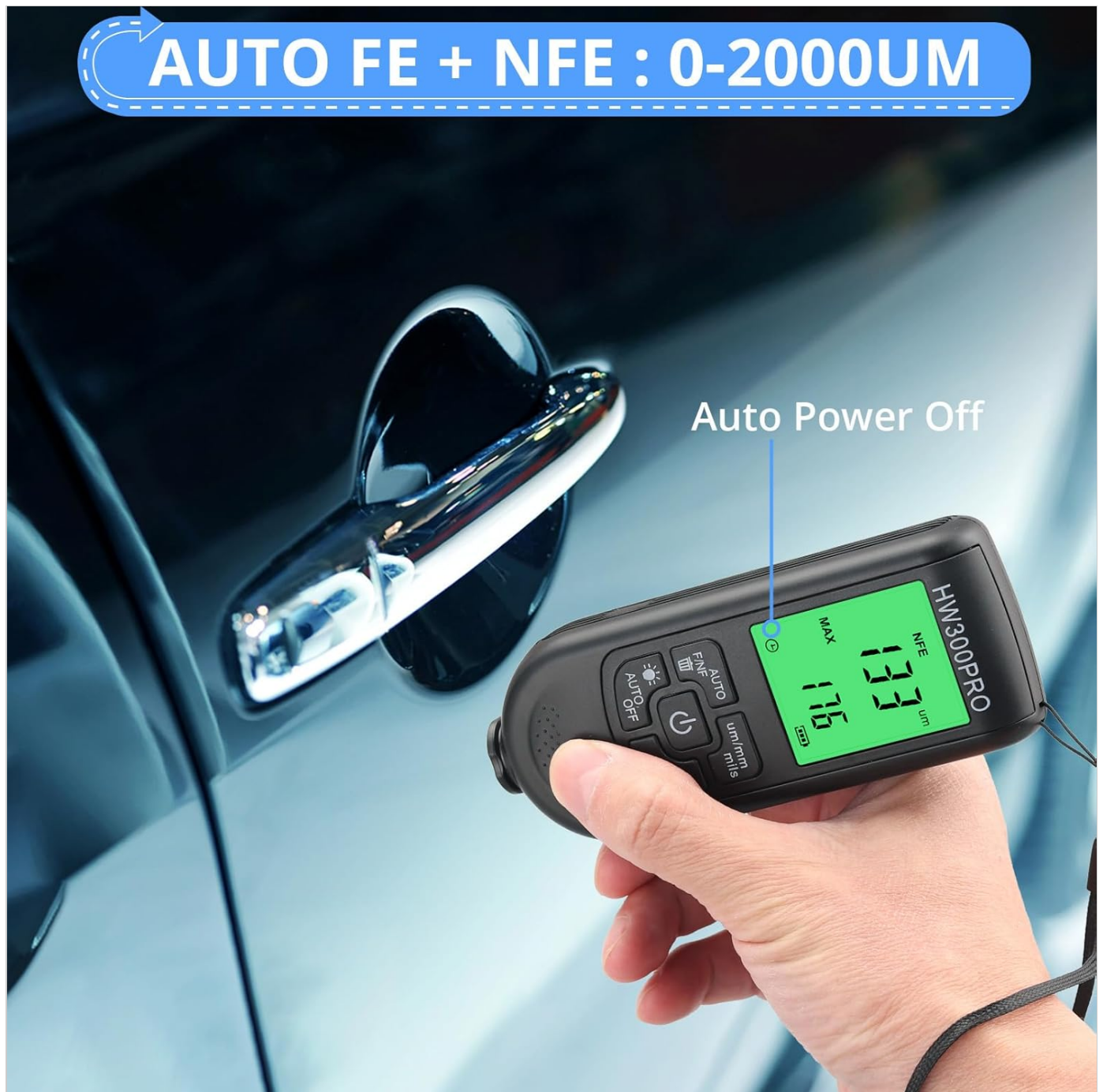
Figure 4.1: Taking a Measurement. The image demonstrates how to position the gauge's probe on a car surface to obtain a thickness reading.
