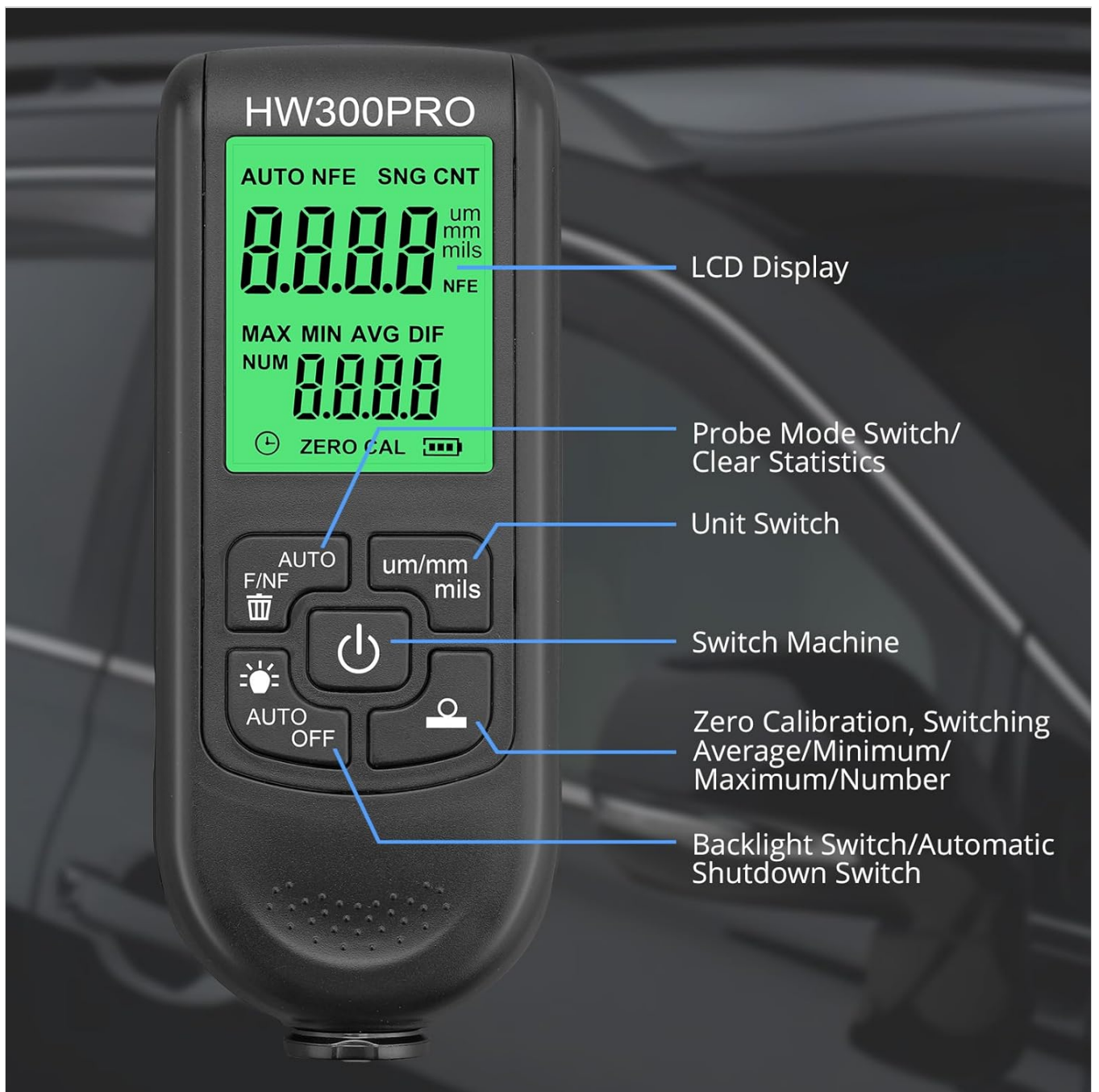
Figure 2.1: Device Layout. This image displays the CAMWAY HW300PRO Paint Thickness Gauge with its LCD display, control buttons, and probe. Key labels include "LCD Display", "Probe Mode Switch/Clear Statistics", "Unit Switch", "Switch Machine (Power Button)", "Zero Calibration, Switching Average/Minimum/Maximum/Number", and "Backlight Switch/Automatic Shutdown Switch".
